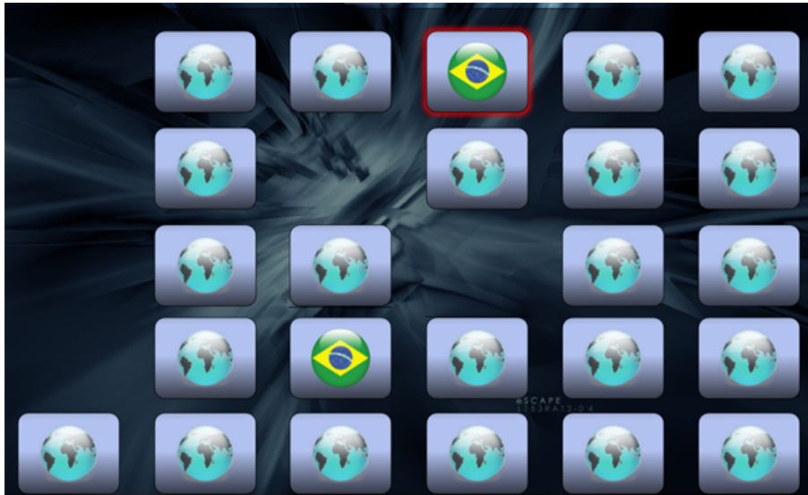
Fig. 7 The GazeMemory game. The objective of the game is to find matching pairs of cards. By fixating a card its content is revealed. When a matching pair is found the cards are removed from the “table”. The prototype is using the Dwell Button component.
