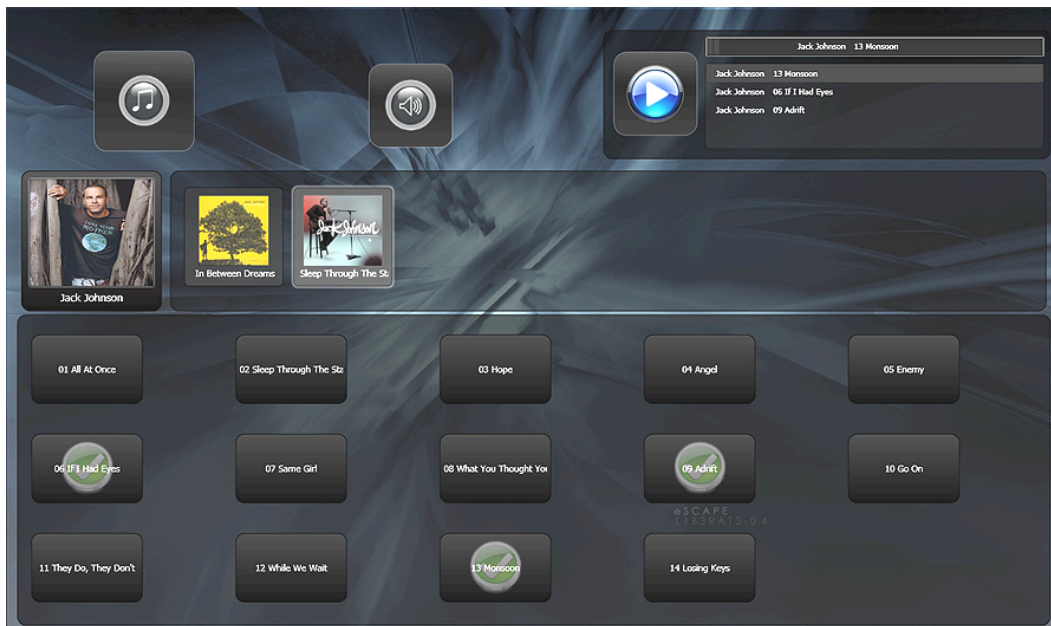
Fig 11. The album and song selection view. By using the Binary Choice components songs can be selected and deselected. This lets the user build a playlist (upper right) By looking at the album covers the list of songs instantly changes (no dwell) The button with a note icon is a Dwell Button that returns to the artist view.
