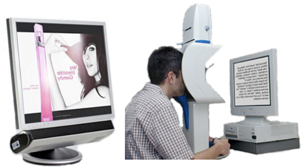
Fig2. Remote based system (left) and high-speed system (right) (Images courtesy of SensoMotoric Instruments)
