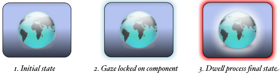
Fig. 3 Dwell Button. The visual indication of the dwell progress. Upon gaze entering the component a thin blue border appears around the button. The icon in the center (globe) is surrounded by a glowing white circle, increasing in size as the dwell progress progresses. When the dwell is completed a thicker colored border appears around the button.
