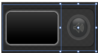
Fig. 5. Binary Choice, the target area (right box) is larger than the actual saccade/selection icon. It raises the tolerance for jitter by reducing the effect of noise from eye tracker
